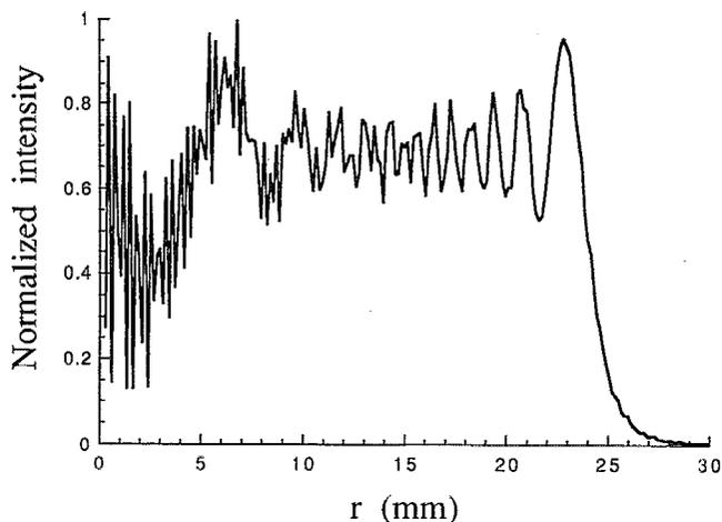
FIG. 2. The calculated intensity distribution at the plane of the second diffractive optical element.
