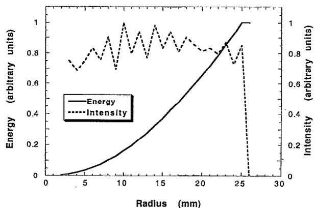
FIG. 5. Relative power  $E(r)$  contained within a circle of radius  $r$  (solid curve) and the corresponding intensity distribution  $I(r)$  (dashed curve) measured at the output plane.
