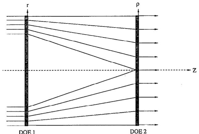
FIG. 1. Optical arrangement consisting of two diffractive optical elements for transforming an annular laser beam into a uniform one.
