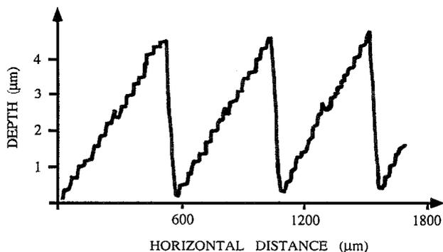
FIG. 3. A surface profilometer trace for a typical section of the diffractive optical element.
