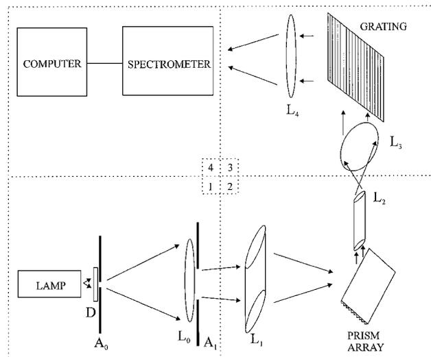
Fig. 1. Experimental optical arrangement for our high-resolution spectrometer: 1–4, building blocks; D, diffuser; A<sub>0</sub>, A<sub>1</sub>, apertures; L<sub>0</sub>–L<sub>4</sub>, lenses. The arrows mark the ray paths through the optical system in the  $x$ – $z$  plane.
