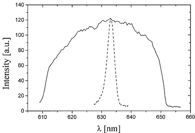
Fig. 4. Measured spectral impulse response of the homemade spectrometer with (solid curve) the anamorphic concentrator and (dashed curve) without it. The FWHM resolution is 2.8 and 36 nm with and without the concentrator, respectively.
