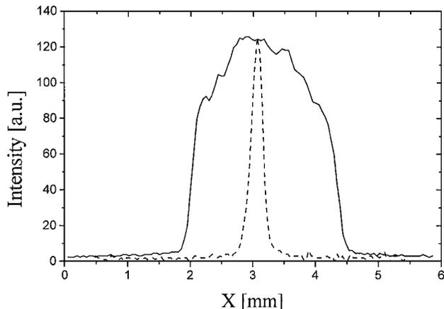
Fig. 3. Measured light-intensity distributions at the output of the anamorphic concentrator (dashed curve) and at the back focal plain of  $L_1$  (solid curve).
