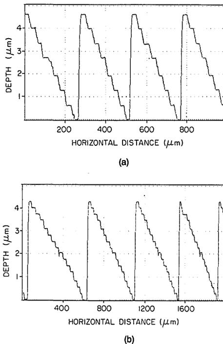
Fig. 4. Surface profilometer traces for typical etched sections: (a) 8 levels of the reflective element, (b) 16 levels of the transmissive element.
