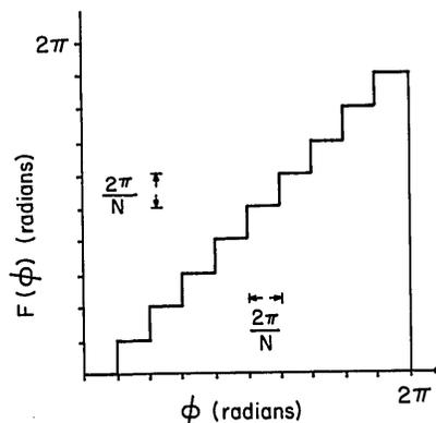
Fig. 1. Actual quantized phase  $F(\phi)$  as a function of the desired hologram phase  $\phi$ .
