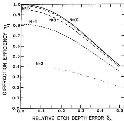
Fig. 2. Diffraction efficiency  $\eta_1$  as a function of the relative etch depth error  $\delta_d$  for  $N = 2, 4, 8, 16$ , and infinity step levels.
