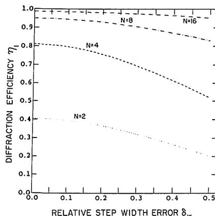
Fig. 3. Diffraction efficiency  $\eta_1$  as a function of the relative step width error  $\delta_w$  for  $N = 2, 4, 8$ , and 16 step levels.
