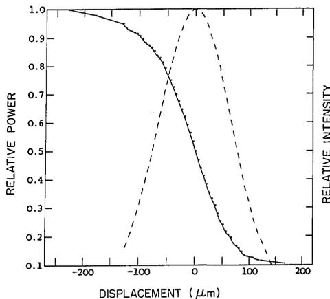
Fig. 5. Relative power of the light as a function of the displacement of the knife edge (solid curve) and the corresponding intensity distribution (dashed curve).
